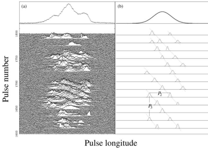
(a) Single pulses from PSR B1944+17 observed with the Arecibo telescope at 430 MHz showing drifting subpulses. (b) Schematic view of the drifting subpulse phenomenon showing periodicities  $P_2$  and  $P_3$ . Taken from "Handbook of Pulsar Astronomy" by Lorimer & Kramer.
