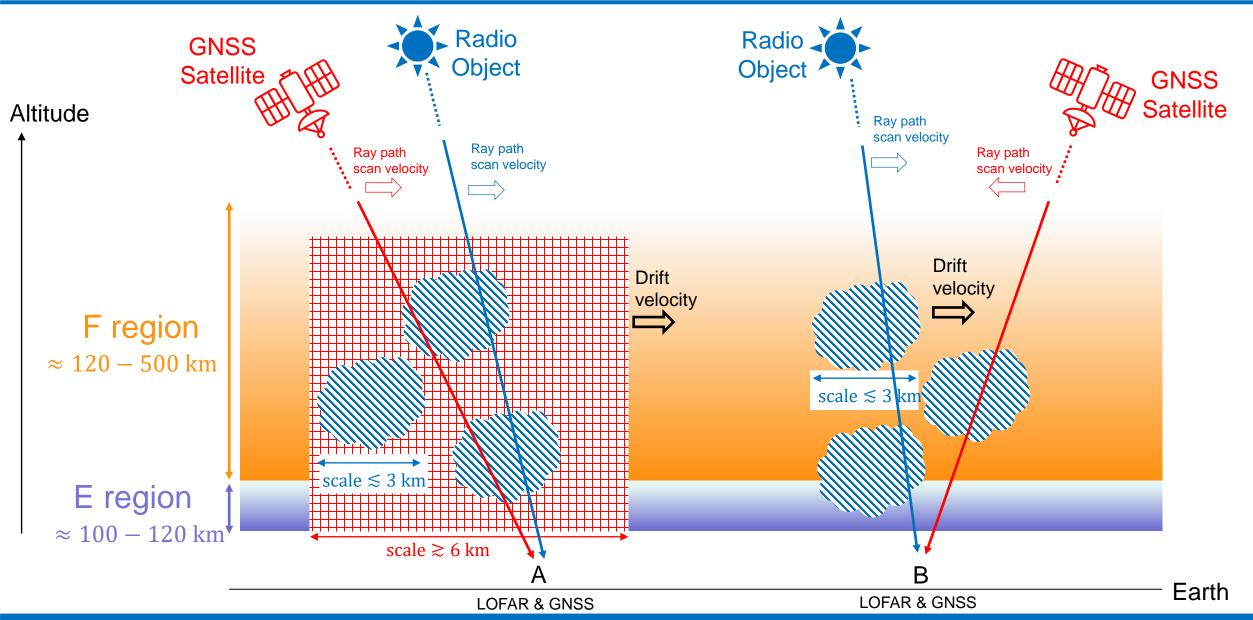
The radio wave scintillation mechanism
